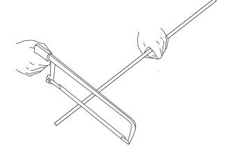
3. Now that the cover tube is cut to 31", measure the all thread tube to be 31 and 3/4" long. And place a mark, with a marker or tape.
