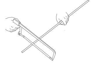
3. Now that the cover tube is cut to 1", measure the all thread tube to be 14 and 1/2" long. And place a mark, with a marker or tape.
