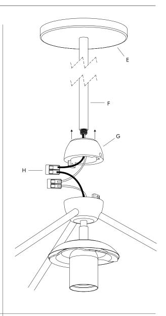
9. Secure the two half hubs together using a hex key and the provided #6-32 socket screws on either side.
