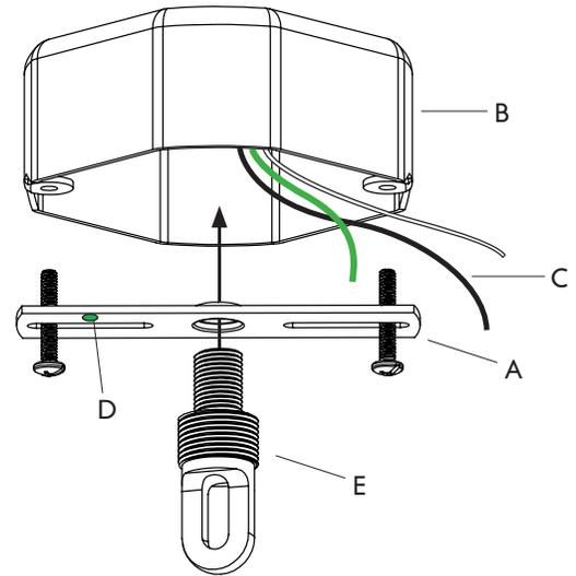
4. Unscrew the hangstraight nut (F) from the hangstraight. Feed onto wire from fixture, followed by the canopy. Carefully raise fixture to ceiling and hold, while guiding the lead wire through the hangstraight into the junction box.
