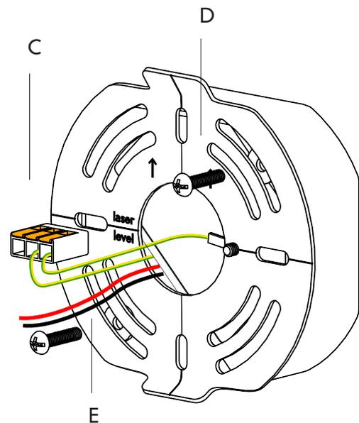
3. Pull the output driver wires (E).
