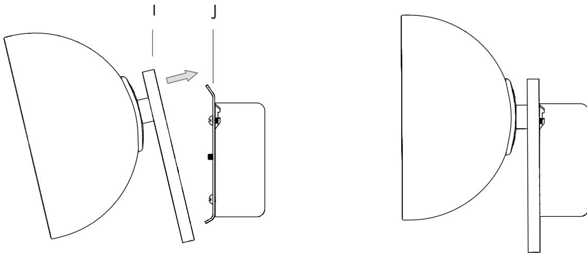
6. Once the fixture assembly is resting in place, use the provided Hex Key (K) to tight the bottom set screw to the crossbar until the backplate is secured.
