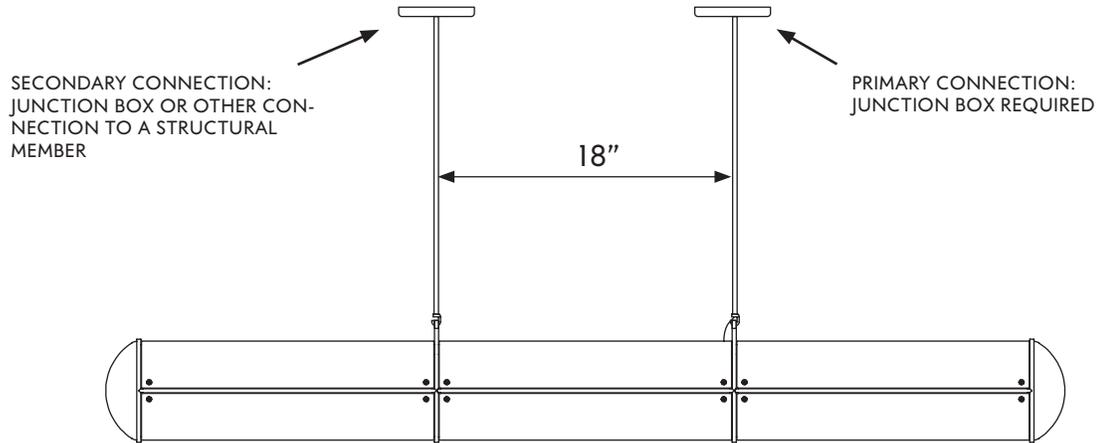
Standard 5 unit configuration with hanging points separated by 3 units:
