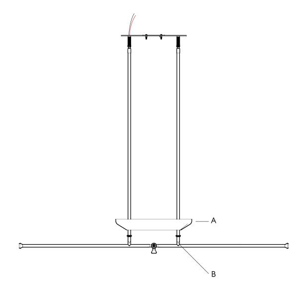
06. Make the electrical connections between the lead AC wires and the driver using the provided Wago Connectors (A)
