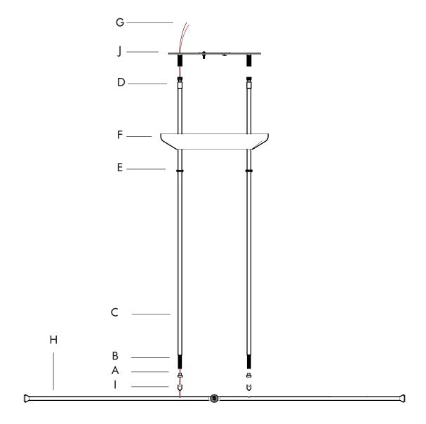
04. Place the crossbar assembly (A) against the two rods and hangstraights (B). Thread the rods (C) down onto the hangstraight until it is flush at the top of the mounting bracket. Secure the stems by threading the two nuts (D)
