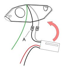
07. Bring the secondary wires and the main ground wire out from the ceiling through the center hole of the crossbar assembly. Connect a Wago Connector to wire. (B)
