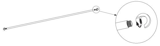
2. Attach the stem (A) to the lighting fixture (B)using the hook and loop. Feed the black lead wire (C) up from the fixture through the stem.
