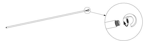
2. Feed the black lead wire (C) up from the fixture through the top of the stem. Attach the stem (A) with connected hub cap (B) to the Astral hub (D) by screwing three screws into place.
